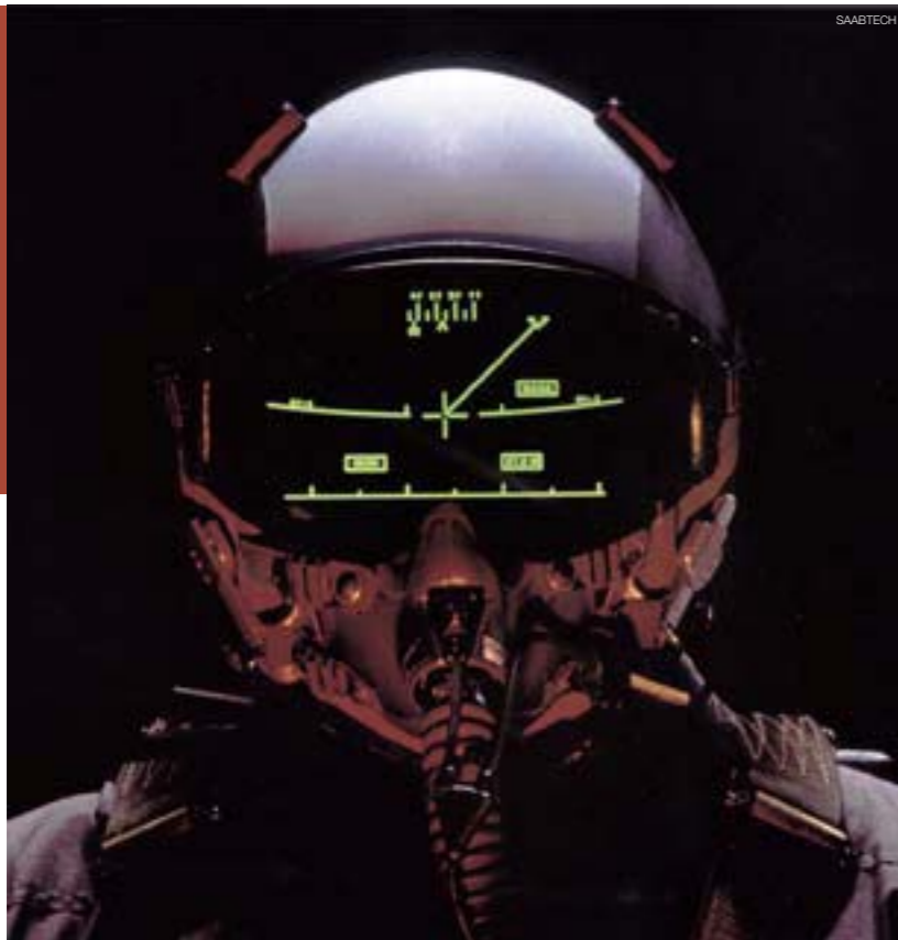
The sight (cross hairs) and relevant information are projected onto the inside of the helmet's visor.
