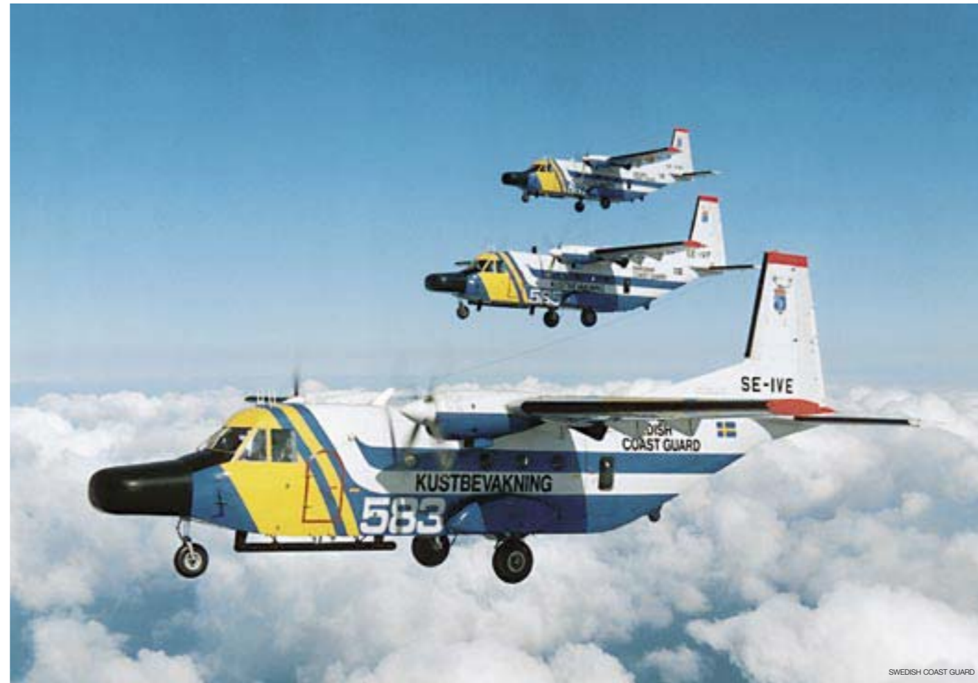
With SLAR radar (Side Looking Airborne Radar) the Swedish Coast Guard can search for oil spills over large areas. The radar covers an area of over 15,000 square kilometres. An oil slick can be seen in the picture.
