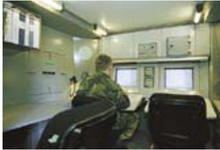
Underrätelseenhet 23 is designed to be manoeuvred by an intelligence officer and a radar operator. There is a third position available for an operator such as an area target officer. All personnel sit in anti-splinter cover.
