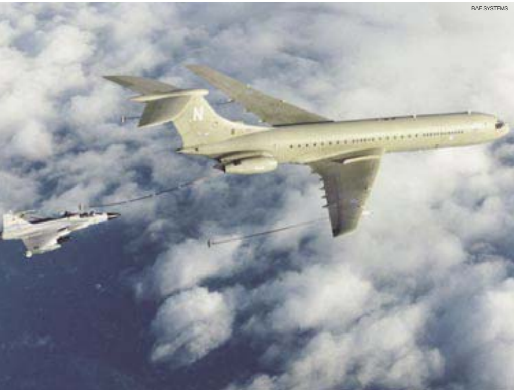
The Hungarian Gripen aircraft will, just as the later Swedish aircraft, be equipped with a retractable air-to-air refuelling probe for fuelling from other aircraft.
