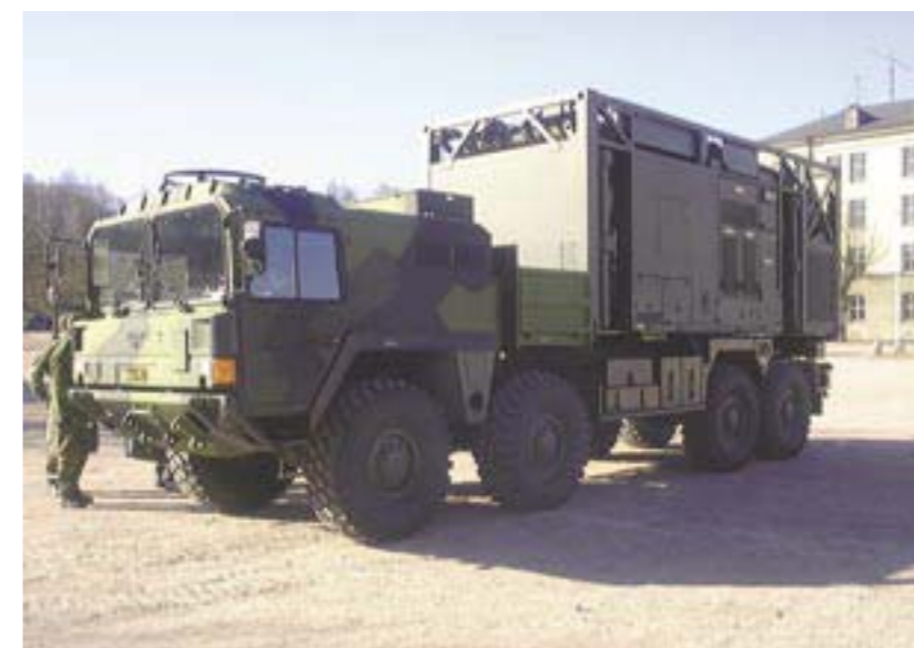
The UndE23 prototype, which has already been delivered to FMV, is based on a Scania truck, but MAN trucks will be used when the actual delivery starts, as they have much better cross-country properties.
