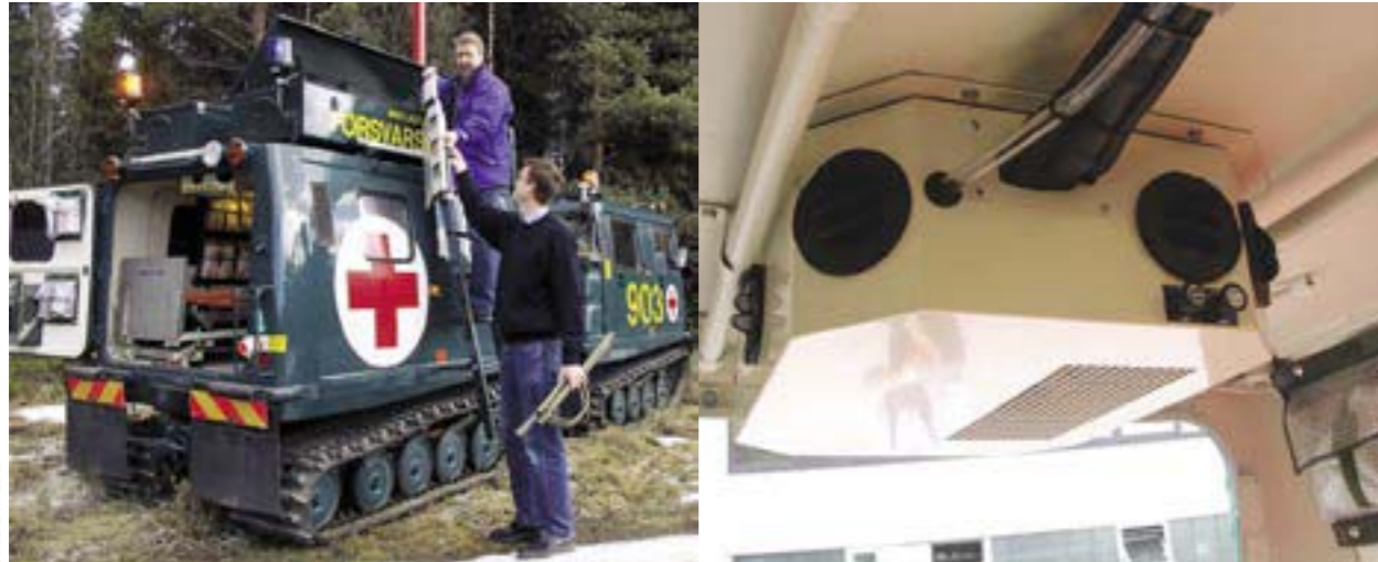
Project manager Johan Åqvist (on the ground) is handed parts of a stretcher by Thomas Olsson, AerotechTelub. Cooling and heating systems ensure a constant temperature of 20 degrees in the vehicle, whether it is +40 or -40 outside.
