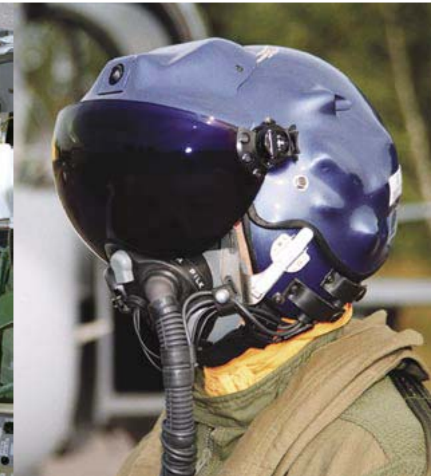
The Guardian helmet offers advanced technology and good precision, but weighs a whopping 1.8 kilos. This, plus powerful G forces, has been shown to put a real strain on the pilot's neck. Guardian was last test flown in Gripen in summer 2002.
