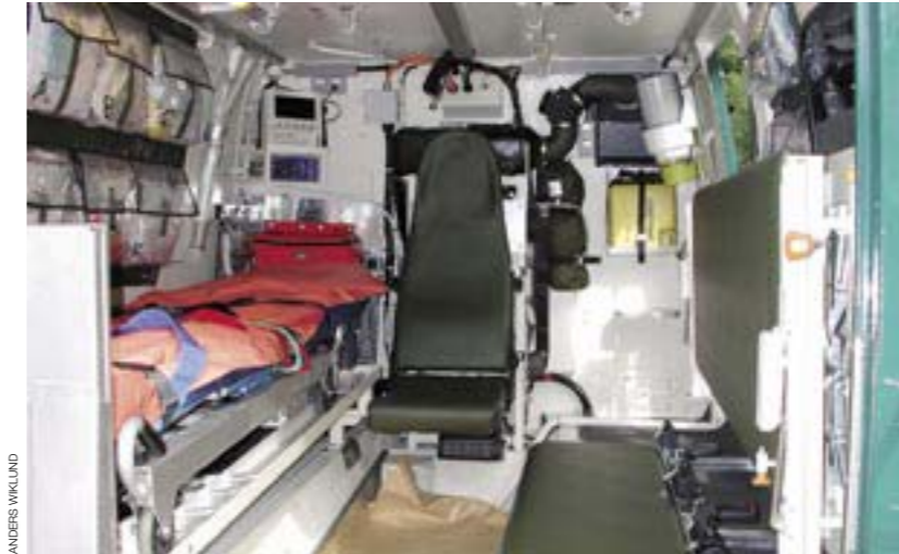
As the rescue caterpillar "Räddningsbandvagn 2077A" is mainly used out in the field, it has a medical equipment level superior to that of a civilian ambulance.
