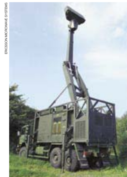
UndE23 has the Anti-Aircraft Artillery's first 3D search radar, which means that the system can detect the distance, direction and altitude of a target.
