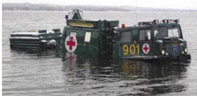
Oh, and it even floats. 2077A is completely water-tight and can be driven in the water. The rescue trailer contains items such as 2x70 kilos of fire-extinguishing powder and spades.
