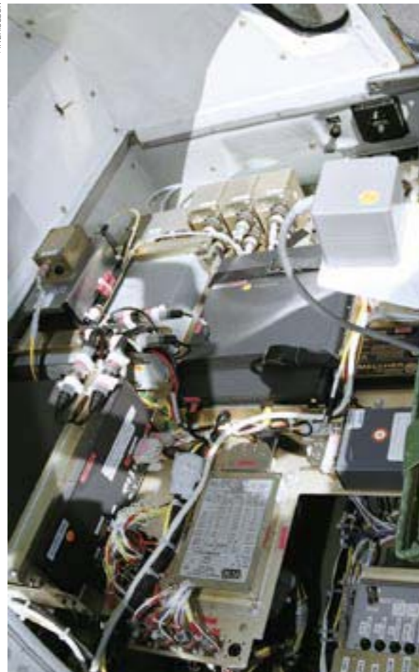
200 kilos of electronics. The Flight helmet's solid test platform for the SK60 aircraft.
