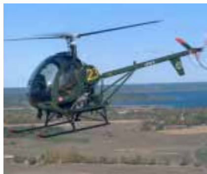
HELICOPTER 5. Hughes 269A/Hughes 300C/Schweizer 300C. Mtow. 930 kg. 28 in the Army. 1962-2002. Fire command, observation, training.
