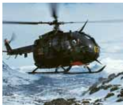
HELICOPTER 9. MBB BO 105 CS. Mtow. 2.5 tonne. 1985-2008. 21 in the Helicopter Wing. Was armed for anti tank missions up to the year 2000. Also transport of troops and materiel. Expected to be withdrawn in 2008.
