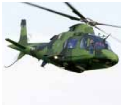
HELICOPTER 15. Agusta A109 LUHS. Mtow. 3.2 tonne. 2005-? (Two provisional helicopters 2002-2006), 20 ordered, 12 land based, 8 ship based (Visby).
