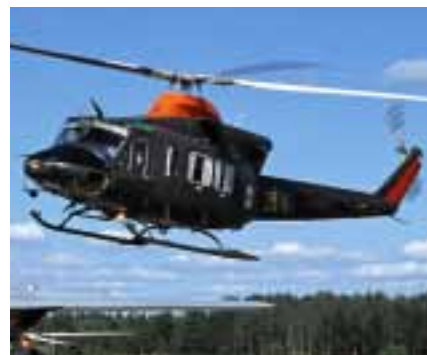
HELICOPTER 11. Agusta Bell 412HP. Mtow. 4.5 tonne. 1994-2004. 5 in the Army. Ambulance missions and troop transport.
